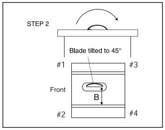
Figure 27. Shim procedure diagram B.
